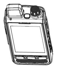
3.Press and hold the power button until the screen lights up (about 3 seconds). Press the power button to put the terminal to sleep, press again to wake it up.
